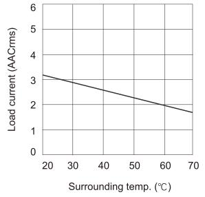
Derating curve is used for finding max. load current at an elevated ambient temperature. When used at full load current, the relays must be placed vertically. If more than one relay Is mounted, please allow a minimum distance of 20 mm in between for sufficient air cooling.
